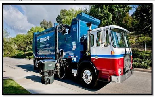
**Front-Loader:** Primarily used to collect 1-8 cubic yard bins from commercial and multifamily customers.
