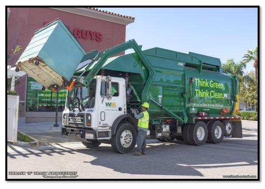
**Rear-Loader:** Rear-Loaders can collect both carts and 1-2 cubic yard bins, as well as public litter cans, bags and bundles of extra yard trimmings and recyclables, and other containers and materials that have to be collected manually.
